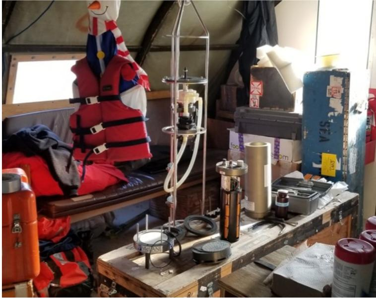
WTS-LV disassembly for cleaning and battery replacement at Bonney camp.
