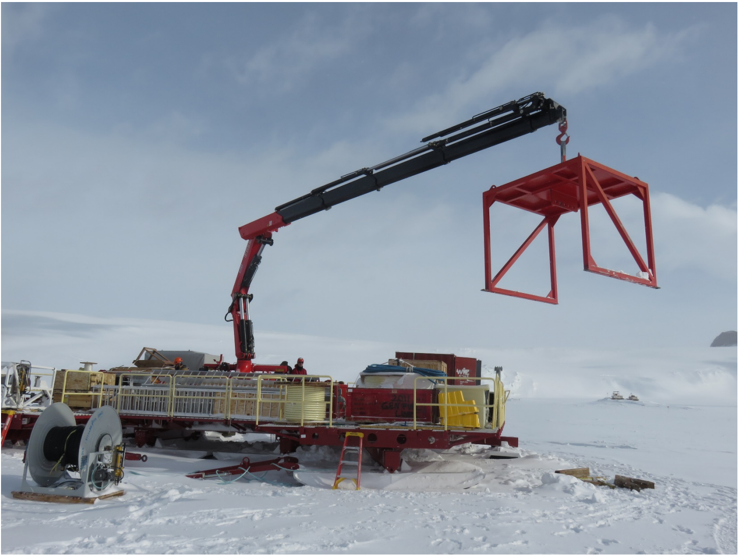
Fassi crane removing load transfer cage from LARS deck.
