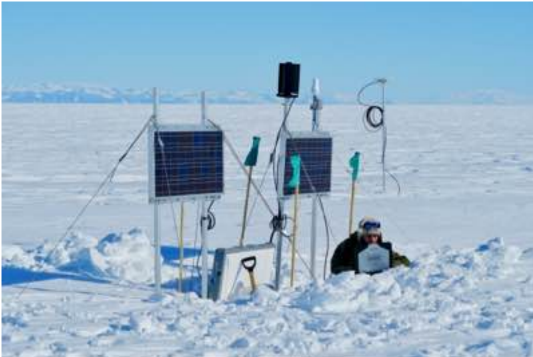
Matt works on reconfiguring the GPS receiver, oblivious to the scenery behind him.
