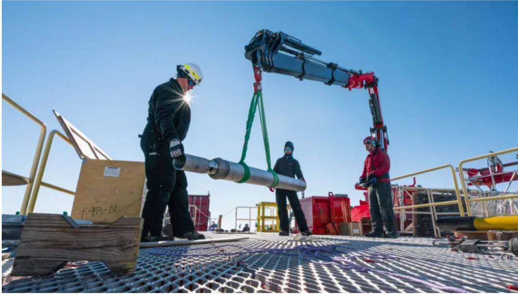
SALSA team members test a gravity corer designed to collect lake bottom sediment samples up to 20 feet deep.
