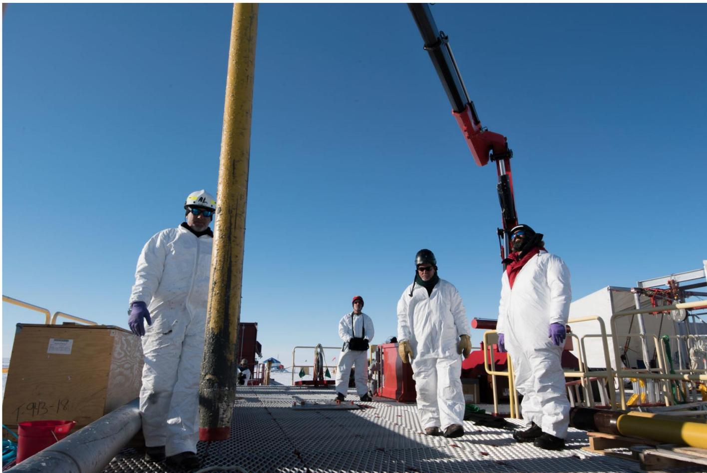
SALSA Scientists lowered a gravity core to the bottom of the Mercer Subglacial Lake in Antarctica to retrieve mud from the bottom.
